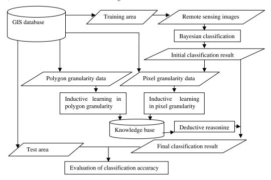
Figure 1. Flow diagram of remote sensing image classification with inductive learning
