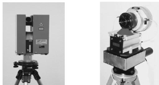
Figure 1. Laser scanner IMAGER 5003 (left), panoramic camera EYESCAN M3 (right)
