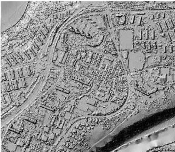
Figure 8. Shaded relief of the laser point cloud.
