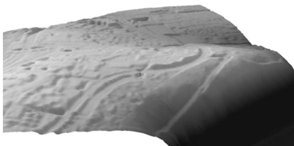
**Figure 13.** Shaded relief of Digital Terrain Model (DTM) with enhanced streets.
