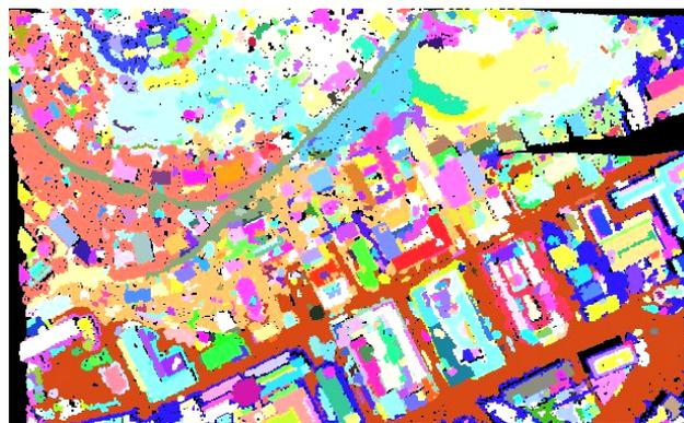
**Figure 2.** Results of the segmentation by normal direction and height differences
