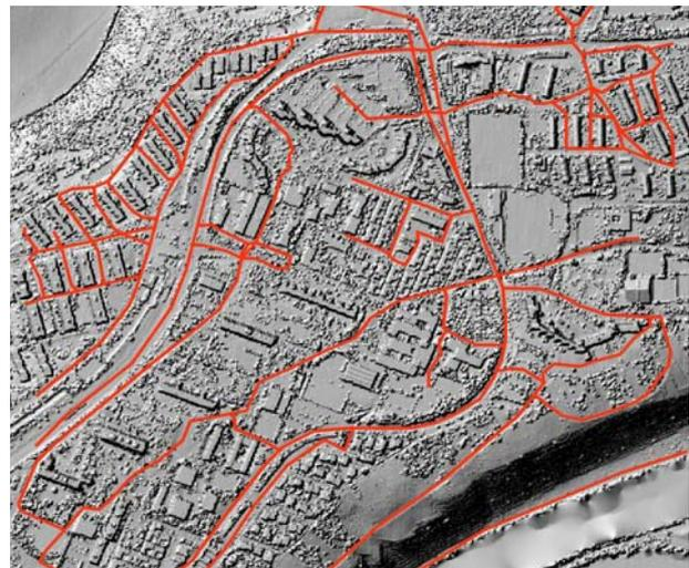
Figure 11. The extracted road network overlaid on the laser point cloud (red-road centerlines, background- shaded relief of the laser point cloud).
