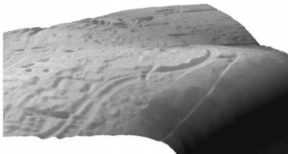
**Figure 12.** Shaded relief of the filtered Digital Terrain Model (DTM) in original appearance; (top) – top view of the filtering result, (bottom) – perspective view.
