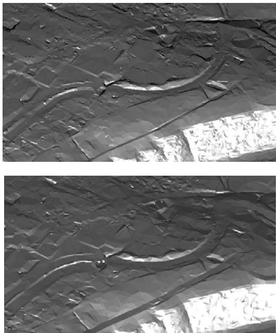
**Figure 5.** DTM with original roads (top) and broadened roads (bottom)
