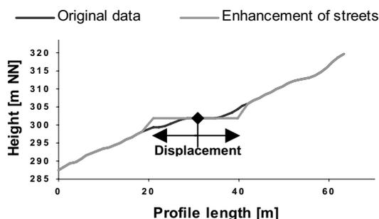
**Figure 6.** Cross-section of the original DTM with and without the enhanced street.
