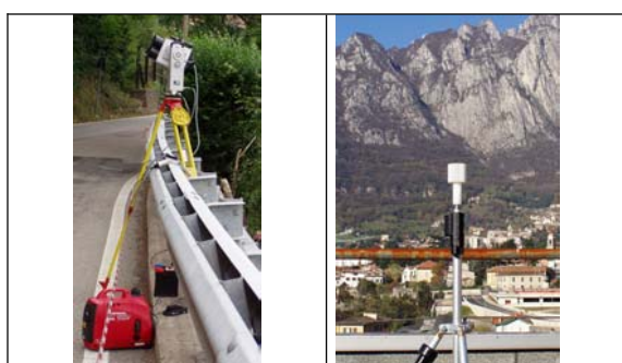
Fig. 7 - The laser scanner Riegl LPM-800 HA (on the left) during a stationing in Porto Ceresio, with the electric generator; a multi-directional target (on the right).
