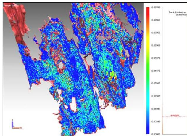
Figure 3: Distances between the full resolution DSM and the DSM at the highest pyramid level; mean = 1.5 cm.
