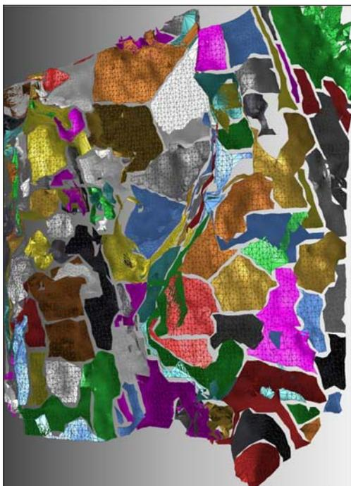
Figure 7: The final segmentation of the DSM: 43 different planes were selected.
