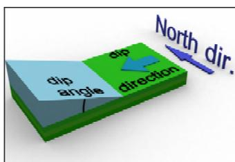
Figure 1: Dip and dip direction of a discontinuity plane.
