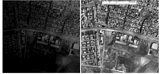
Figure 6: Subset image covered by the smoke plume before (left) and after (right) the radiometric enhancement.
