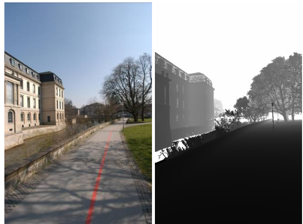
Figure 4. Depth image calculated to fit the original image, left: the depth image, right: the original image. Because the spatial resolution of the laser point cloud is much sparser than the image resolution ( 0.12^\circ compared to 0.03^\circ here) filling of depth image was applied for demonstration purposes only.
