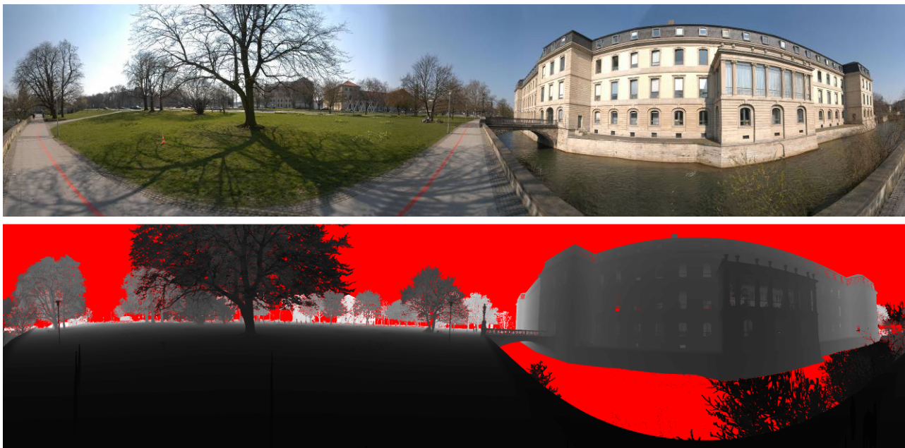
Figure 1. Top: panoramic view of the scanned scene as acquired by a camera mounted on the scanner (for the original images see Figure 5), Bottom: Polar representation of terrestrial laser scans; the horizontal and vertical axes of the image represent the values of \theta , \varphi respectively and intensity values as distances \rho (bright=far). "No-return" and "no-reflectance" pixels are marked in red.
