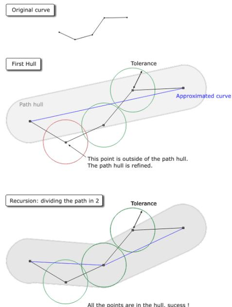
Figure 2. Simplification of laser sections based on Douglas-Peucker.
