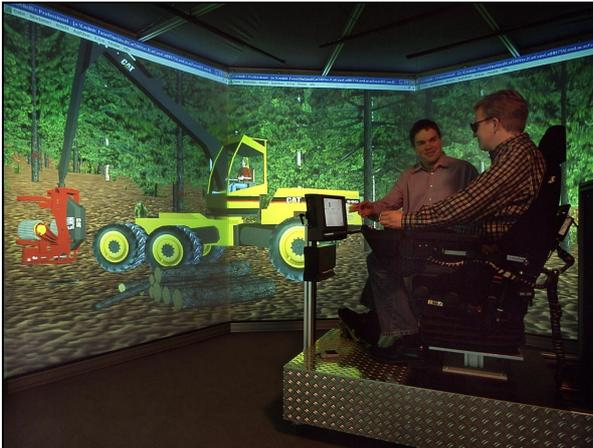
Figure 6. Forest Machine Simulation in the Virtual Forest
