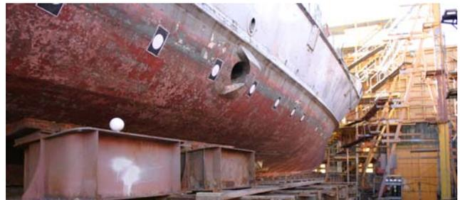
Figure 2. Waterline marked with black and white targets
