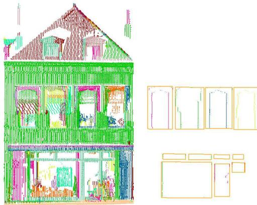
Figure 6. An example showing an extracted window is smaller than reality, as a result of obstacles on this window
