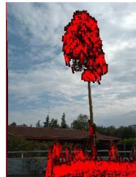
Figure 15. Full-waveform ALS data is superimposed onto the terrestrial image (Litkey et al., 2007).
