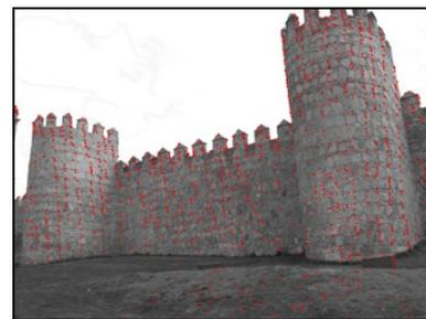
Figure 3. Förstner detector applied to medieval wall.
