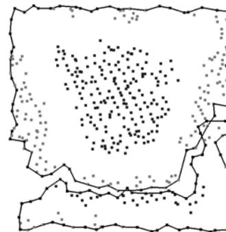
**Figure 9:** Outline of the segments of the nearly flat roof
