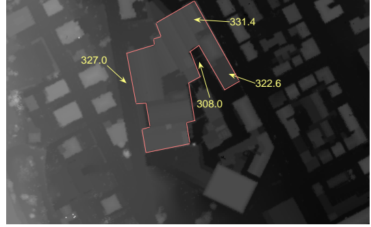
Figure 5: Spacious building block - special case; Height value on the roof in one side (right) is less than the height of the road next to it (left)
