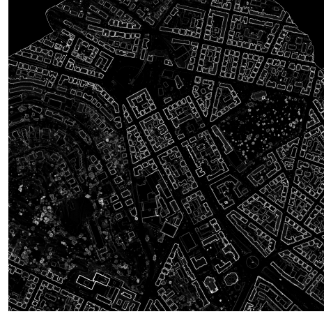
Figure 7: Local Range Variation ( LRV ) image which mainly highlights height jumps in range image
