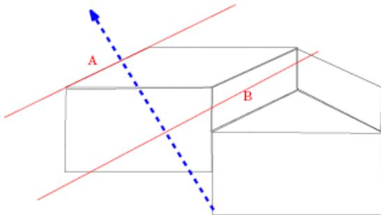
Figure 11: Triangles on roofs A and B projected onto the averaged normal vector (thick dashed line)
