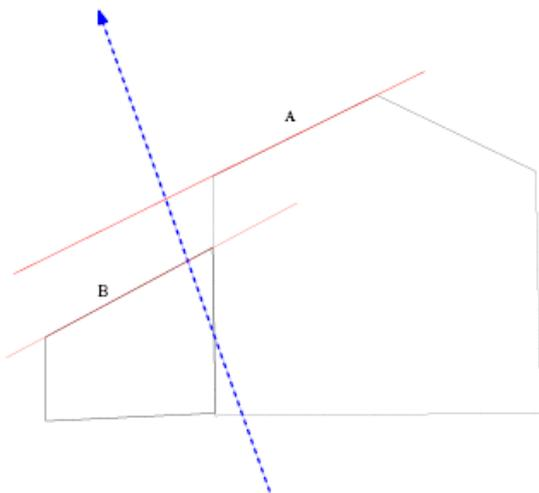
Figure 12: Triangles on roofs are projected on its averaged normal vector (thick dash line)
