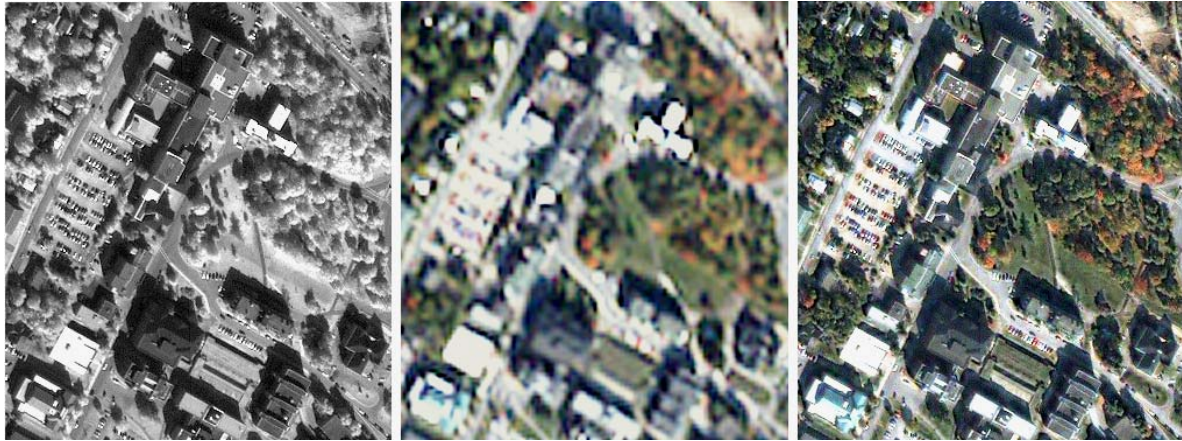
Figure 2. Automatic image fusion of Ikonos Pan and MS images, University of New Brunswick, Canada. Left: Original panchromatic image (1 m); Center: Original natural colour image (4 m); Right: Fused natural colour image (1 m).
