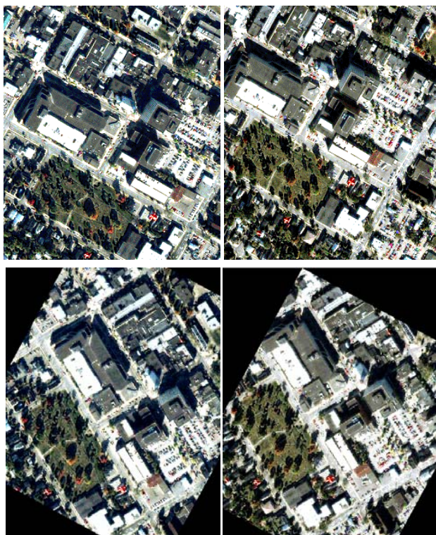
Figure 5. Epipolar geometry resampling. Top: Ikonos image pair before epipolar resampling; Bottom: epipolar images.
