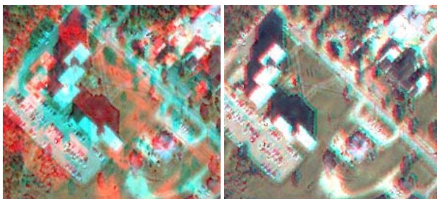
Figure 8. Influence of overall horizontal parallaxes for effective colour 3D viewing. Left: larger overall horizontal parallaxes cause stereo fusion problems; Right: small overall horizontal parallaxes are more comfortable for colour 3D viewing.
