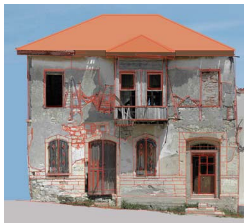
Figure 5. The orthoimage of the southern façade, overlapped with the 2D scaled drawing
