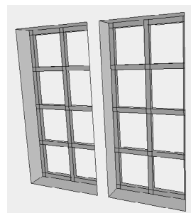
Figure 6. Reconstructed crossbars for two windows.
