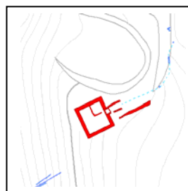
Figure 16. Big water cistern ( castellum aquae ) with pipes referencing.
