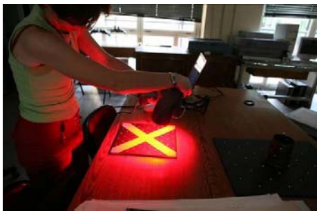
Figure 10 – The geometric calibration of the Handyscan
