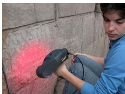
Figure 11 – Example of radiometric calibration of the Handyscan
