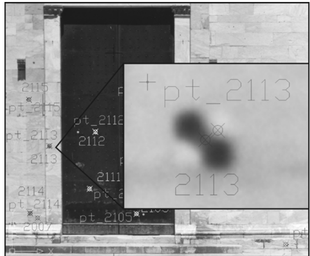
Figure 4 – Laser-computed and topographical targets on rectified image.
