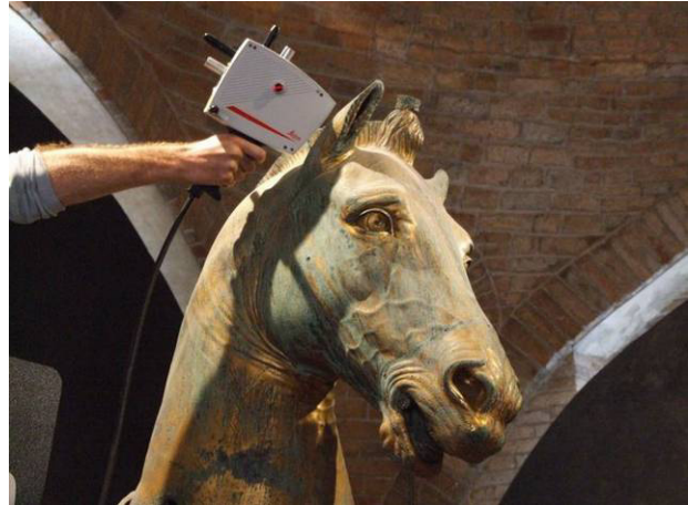
Figure 7: It's possible to see a moment of the scan. The red dot on the side of the hand scanner means that the laser ray hooks up the instruments and that the scan can be done!
