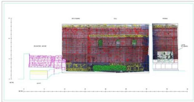
Figure 1 The plotting of the walls with the texture of the orthoimages
