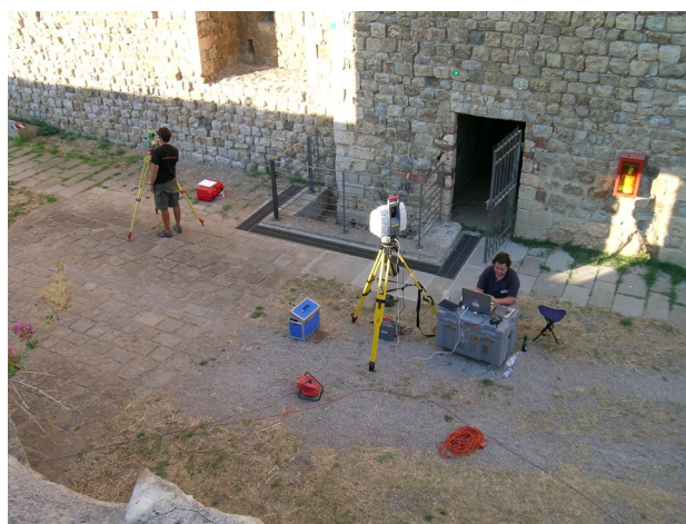
Figure 1. Registration of the targets by the total station and by the laser scanner.
