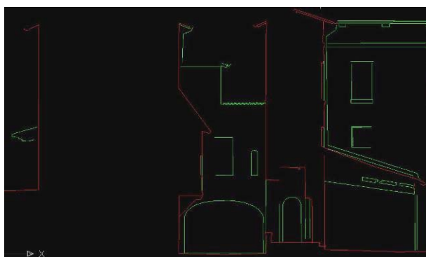
Figure 9. Cross-section and internal front of Rocca realized with laser scanner data
