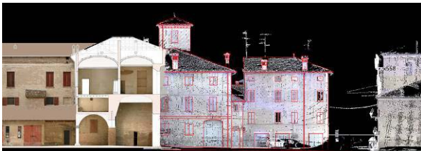
Figure 13. Drawing of the fronts of buildings, from laser scanner points cloud associated with colour information
