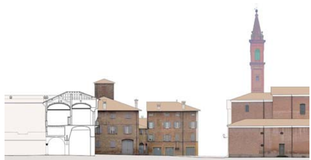
Figure 15. Photo-mosaic of fronts: extraction from laser scanner cloud of points useful to rectify all the images
