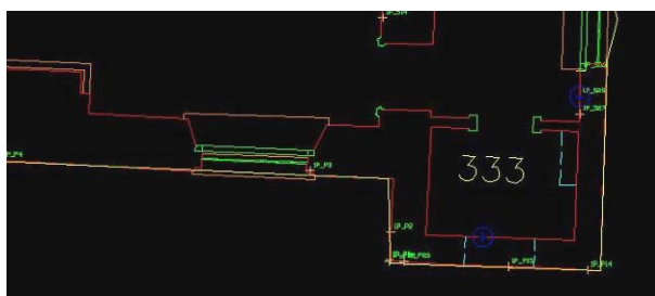
Figure 5. In yellow the horizontal cross-section extracted by laser scanner data; in red the plan realized with manual and topographic techniques
