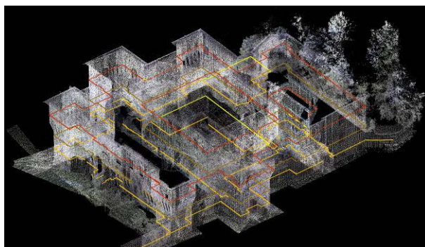
Figure 3. Extraction of four horizontal cross-sections from laser scanner points clouds
