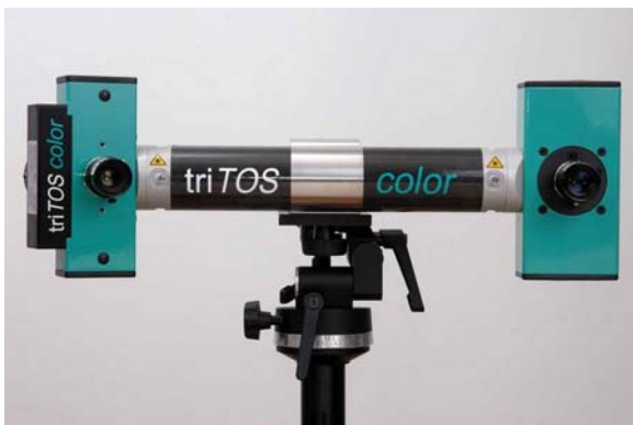
Figure 3. triTOS fringe projection system
