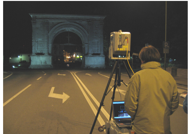
Figure 3. Part of the laser scanner acquisition performed during the night
