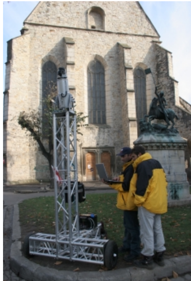
Figure 2. Measuring with RIEGL LMS-Z420i 3D laser scanner
