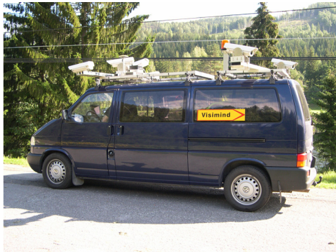
Figure 1. Visimind MMS - the data acquisition hardware, ©Visimind 2007
