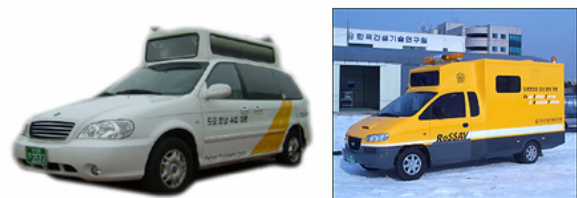
Figure 2. Road imagery acquisition vehicle(Left), Road safety survey and analysis vehicle(Right)
