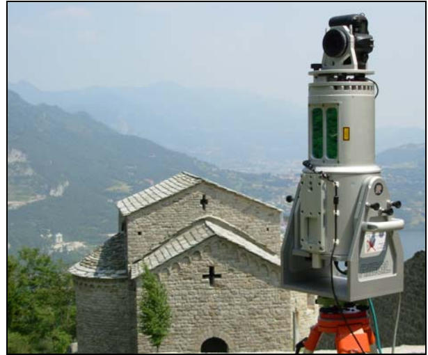
Figure 3: laser scanner Riegl LMS-Z420i with its integrated camera during scanning of the oratorio di San Benedetto roof.
