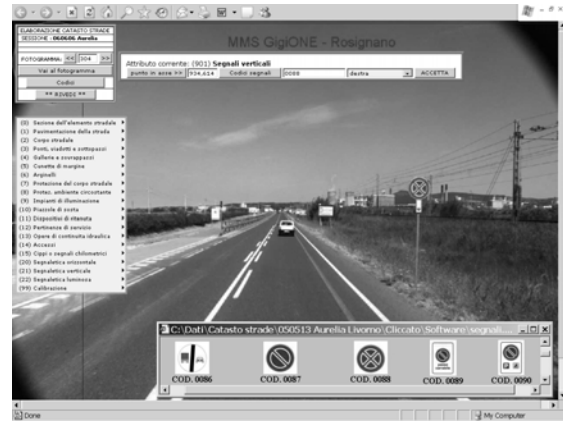
Figure 7. Vertical signs data extraction.
