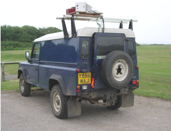
Figure 1. The lidar system mounted on the 4x4 vehicle.
