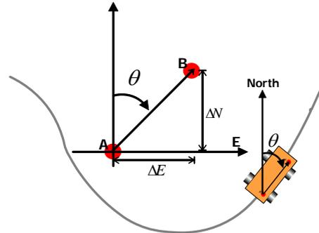
Figure 3: Obtaining GPS heading from the positional differences of two antennas
