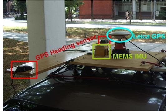
Figure 6: The experimental platform
