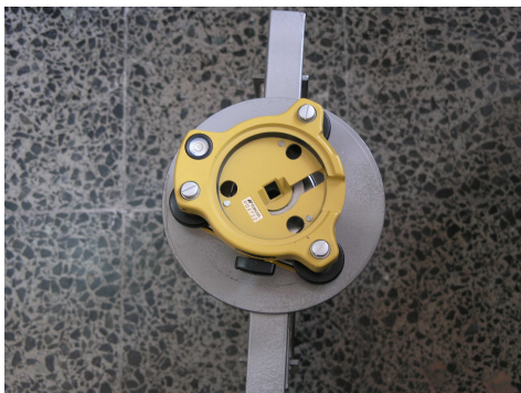
Figure 3: the top view of flat disk fixed on steel bar carrying tribrach with bubble.
