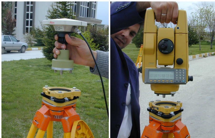
Figure 2: Use of single tribrach (TeT) combination technique for both GPS and EDM
