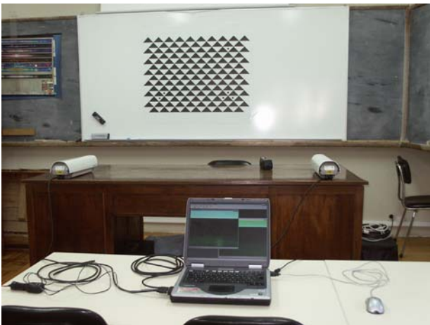
Figure 4: Image acquisition to obtain calibration parameters of the video camera lenses.
