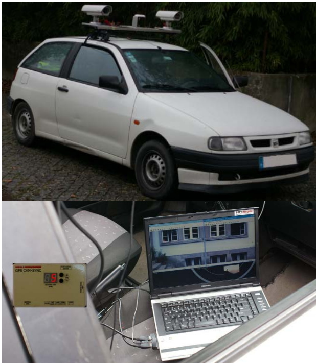
Figure 2: Surveying vehicle and system components.
