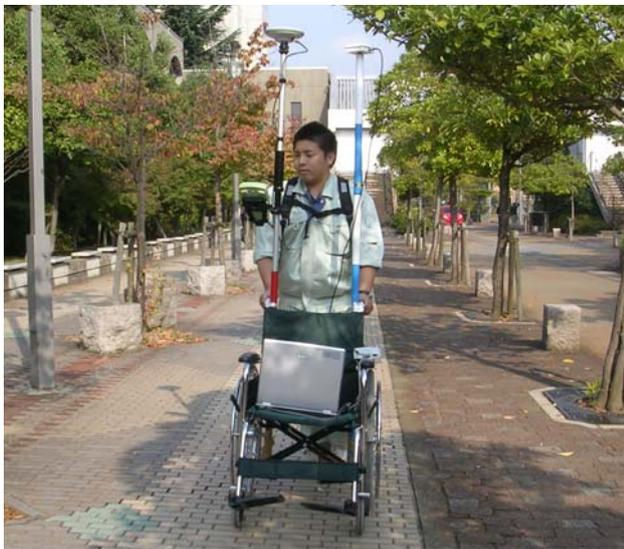
Figure 4. Positioning of D-GPS and VRS-GPS
