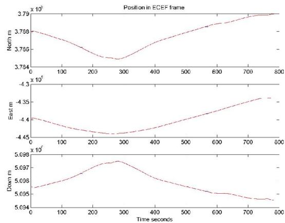
Figure 5. KM filter positions in the ECEF Frame
