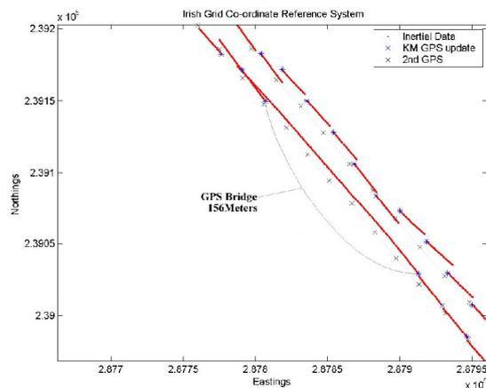
Figure 6. Primary GPS with satellite error (Road Section B)
