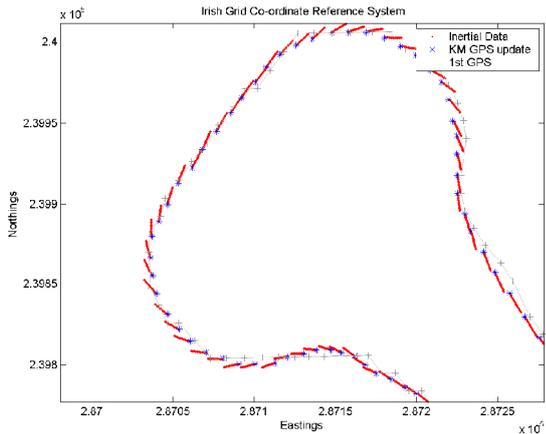
Figure 8. EKF with second GPS Receiver
