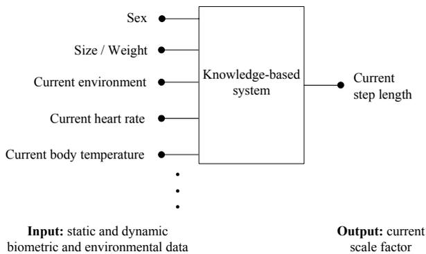
Figure 2. MISO-example for the knowledge-based calibration of the step counter.
