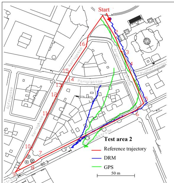
Figure 4. Results from test area 2 without WiKaF.
