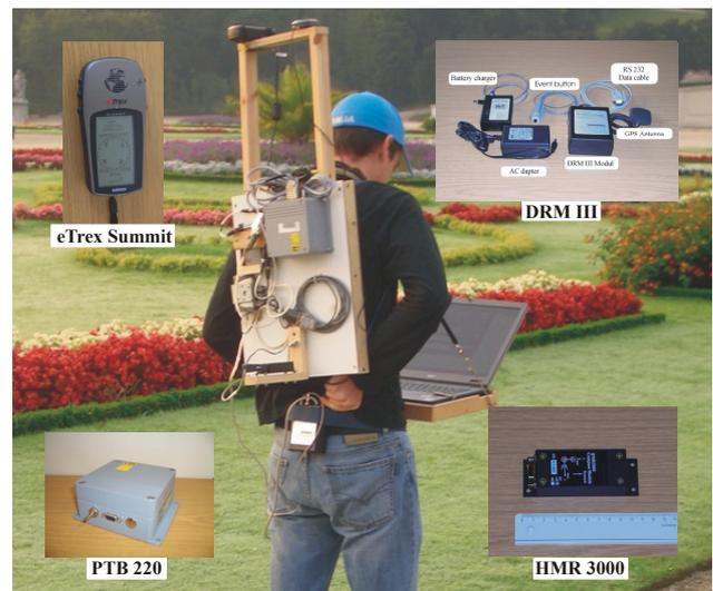
Figure 1. Multi-sensor system from the NAVIO project.
