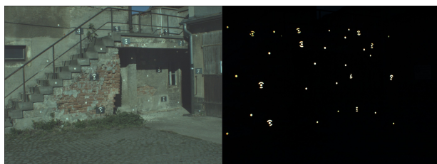
Figure 3. Calibration field with retro reflective targets (left) and Image from the Marlin camera with external illumination
