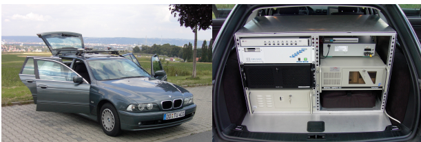
Figure 1. Mobile Mapping car (BMW) of the chair of road design (left) and the view to the server rack (right)
