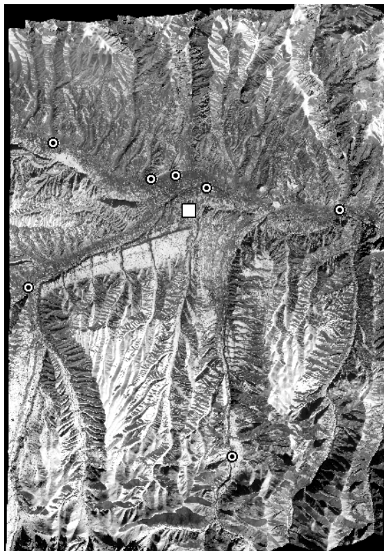
Figure 8: The distribution of the GPS ground control points on the IKONOS image mosaic. In the centre the master station position.
