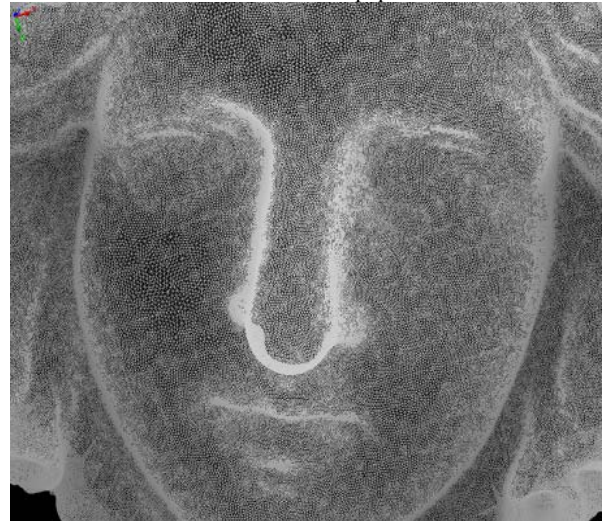
Figure 14: A particular of the surface mesh of the ornament generated using the Leica T-Scan. The size of the shown part is circa 7 cm.
