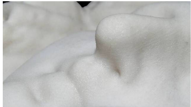
Figure 15: A particular of the prototyped ornament. It is evident the high level of detail of the object. This kind of prototype can be used to build silicone moulds or stamps for wax or sand melting.
