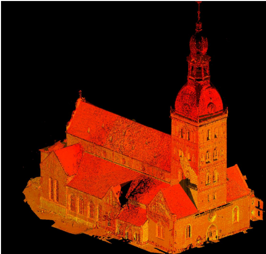
Figure 3. Cathedral 3D Model from point cloud and mesh
