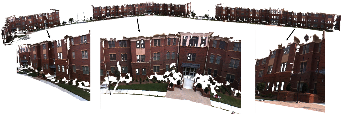
Figure 7: A two-camera reconstruction comprising more than 2,600 frames. Close-ups show that features such as the ground plane which is viewed at an angle from the camera and thin objects such as the light pole on the right are reconstructed well.
