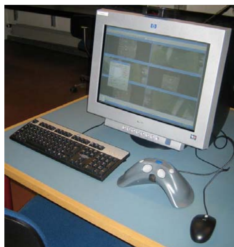
Figure 4: Digital stereoworkstation "Intergraph Image Station SSK"
