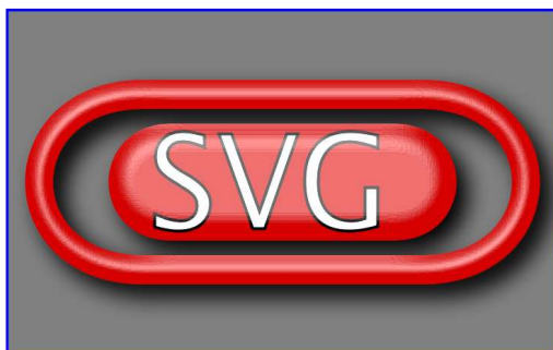
Figure 2: Filter example: combination of a gaussian blur, offset, specular lighting and composite filter, Source: http://www.w3.org/TR/SVG11/images/filters/filters01.svg © W3C consortium
