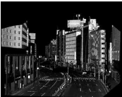
Figure 1: Ground-based LiDAR image of city street (Tokyo).
