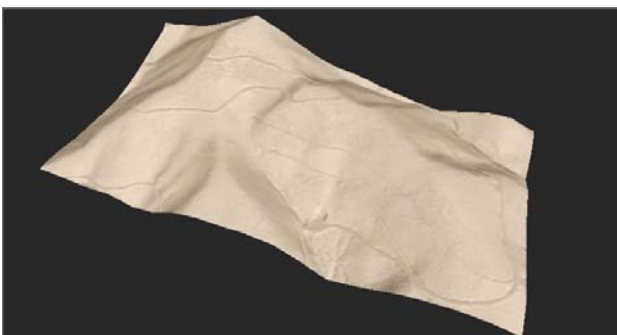
Fig. 7: The illustration shows the calculated DTM of the test area Günterstal in the black forest covered with an artificial texture. The raster resolution is 1m.
