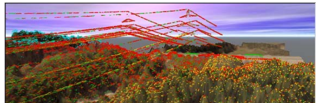
Fig. 9: Engen power supply line above the DSM.
