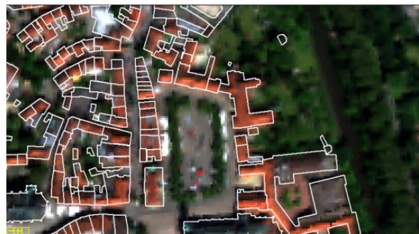
Figure 4. RGB-Image of the HyMap data with overlay of a GIS-Layer (buildings).
