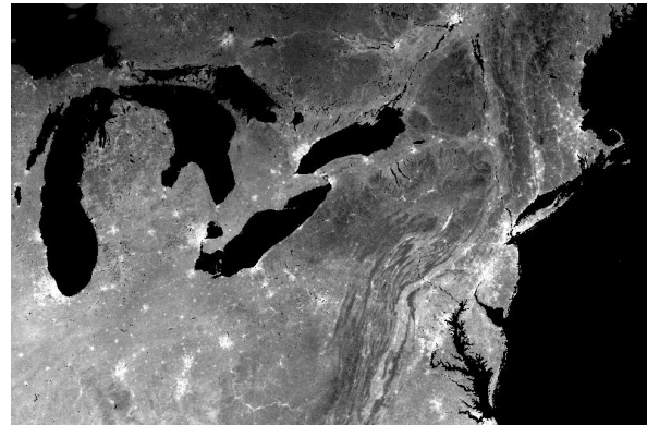
Figure 2. AVHRR channel 3 mean brightness temperature after canopy closure 1997. Bright patches correlate with high concentrations of anthropogenic building materials. Bright lines correlate with highway rights-of-way. Increasingly dark gray tones correlate with increasing canopy density. Note the pervasive pattern of settlements from Virginia to Boston.
