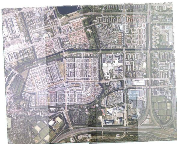
Illustration 2: Ultracam orthorectified images overlay
