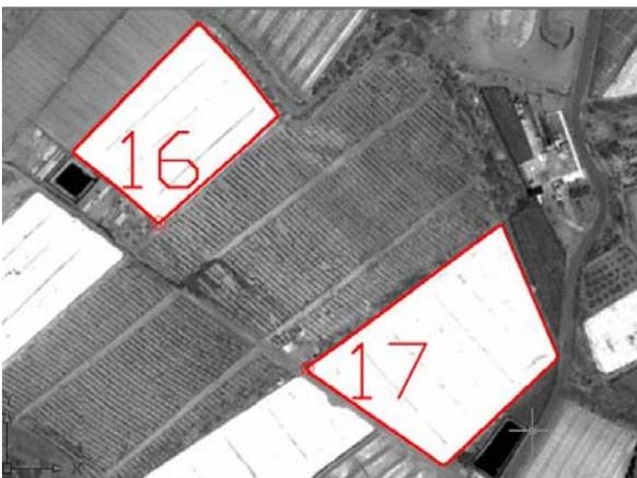
Figure 7. Two points chosen on the vectorial cartography at a scale of 1:1,000 overlaid an IKONOS's orthoimage.
