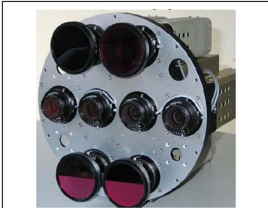
Fig. 7: configuration of UltraCam<sub>D</sub> lenses
