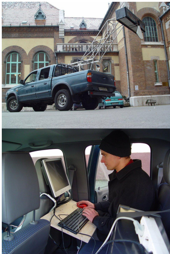
Figure 3. The instrument platform mounted on the pickup and the controlling environment
