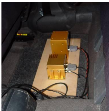
Figure 5. The investigated IMUs (left NAV420CA, right AHRS400CB) and (bottom) the common mount platform
