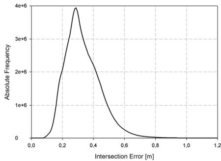
Figure 2. Histogram of intersection error for test area (117 km<sup>2</sup>) covering 6 image tracks over the full width of the survey area.
