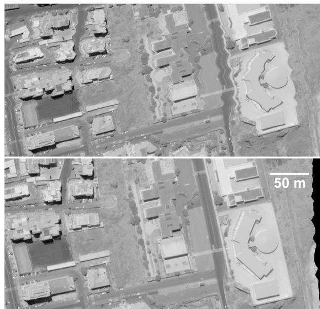
Figure 1. Top: example of unusually strong geometric distortions in the raw nadir image caused by roll angle variations. Bottom: result of geometric image correction.
