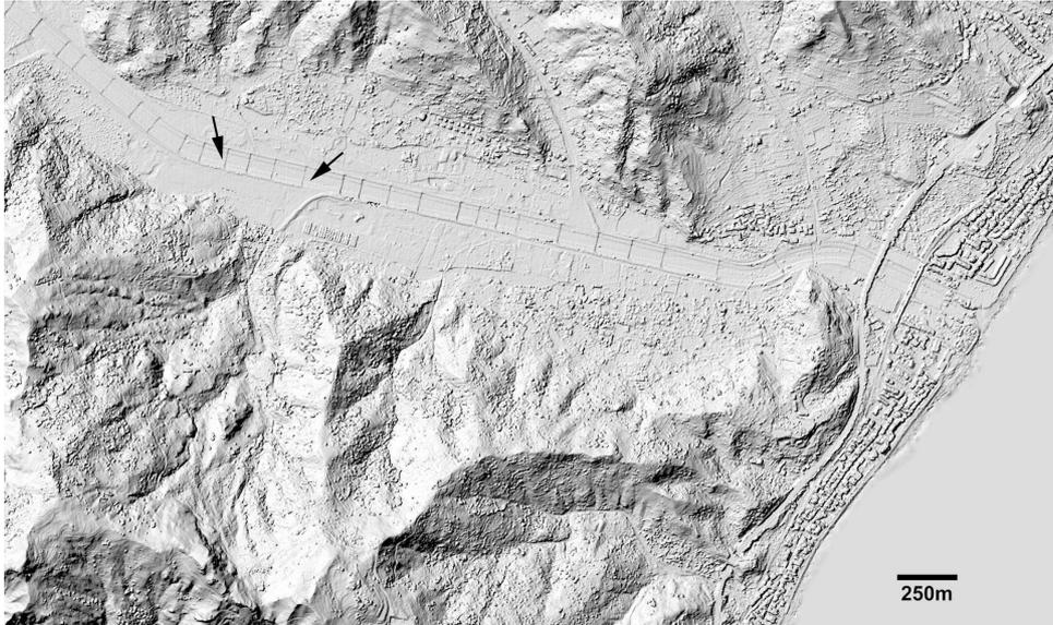
Figure 6. Shaded relief map of a coastal area near Taormina. The small arrows point to engineering constructs which correspond to steps in the river bed approximately one meter high.
