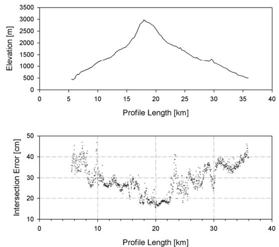
Figure 4 Top: Vertical section crossing the summit area of Mt. Etna in E-W direction. Bottom: Mean intersection error along the section, calculated in 25x25 m grid cells. The significance of local ground resolution is indicated by the inverse correlation between the intersection error and true ground distance.
